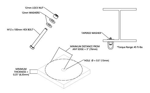
**IMPORTANT:** Use a grade 10.9, grade 12.9 (or equivalent) bolt no shorter than 4" (100mm) with a locking nut and washer in steel applications. When installed, the swivel anchor must be flush with the steel surface.
