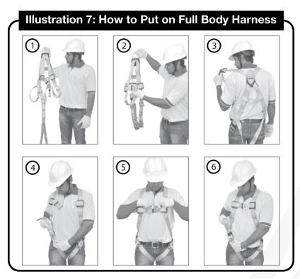
**Step 1:** Hold harness by grasping back D-ring. Shake harness to allow all straps to fall into place.
