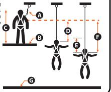
If there is a risk of a fall or if the only anchorage point is below the attachment points on the harness, it is essential to use a lanyard provided with an energy absorber. Before using a shock absorbing lanyard, ensure that there is sufficient fall clearance below the user to prevent any collision with the structure or ground.
